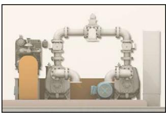
The Gorman-Rupp **Base Mounted Auto-Start** station uses a liquid level control which automatically converts to 12 volt DC and drives the pump with a standby engine providing normal pumping service during power failures. When power resumes, AC motor operation is automatically restored. It meets all standby requirements and uses a variety of fuels.
