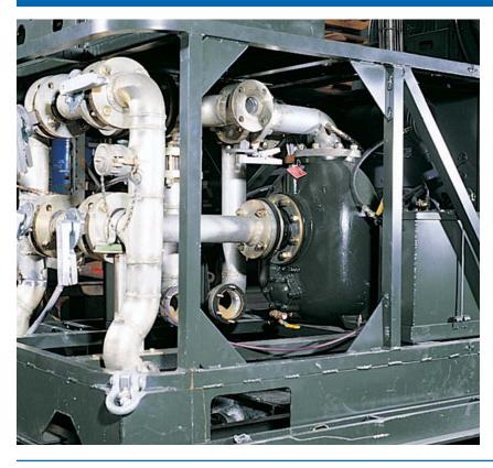
Gorman-Rupp O Series® selfpriming centrifugal pumps have a straight-in suction design which eliminates entrance restrictions and provides better performance when handling a variety of clear liquids.
